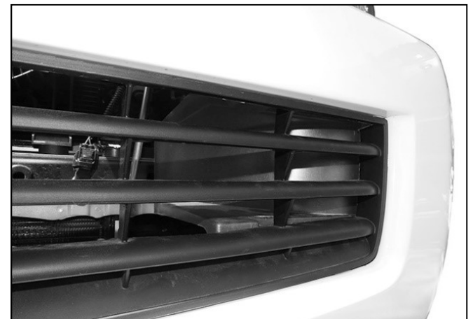
(Fig 5) Models equipped with driver/left side air deflector, cut or remove air deflector to clear the Top Brackets
