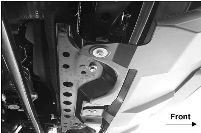
(Fig 2) If necessary, temporarily remove bumper cover hardware to access bumper bracket (passenger/right side pictured from below)
