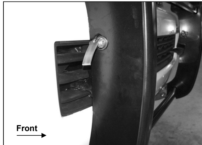
(Fig 17) Pull handle to "open" Quick Release
